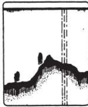
Interference from electrical equipment
